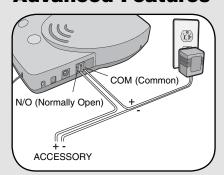
The Base Station has a relay which can activate other devices such as a doorbell, buzzer or light. The relay switch can handle up to 24 Vac at 10 amps. The accessory device will need a separate power supply. The accessories can be purchased at any electronics store.
